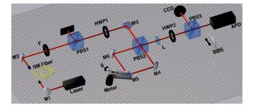
FIG. 1. Experimental setup. The goal is to estimate the deflection of a mirror, represented by g. See the text for a complete description of the experiment.
