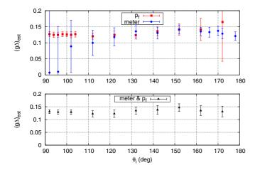
FIG. 6. Estimated value of  $g\Delta$  from the experiment, for postselection in  $|\psi_f\rangle = |\psi_i\rangle$ . Blue circles correspond to estimates from measurements on the meter, red squares correspond to estimates obtained via the statistics of postselection events, and black triangles correspond to estimates using information of both the meter and the statistics of postselection events. Error bars represent 3- $\sigma$  dispersion.
