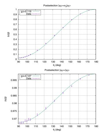
FIG. 2. Measured postselection probability as a function of the initial polarization state for strategies  $|\psi_f\rangle = \hat{\sigma}_3 |\psi_i\rangle$  (top) and  $|\psi_f\rangle = |\psi_i\rangle$  (bottom).
